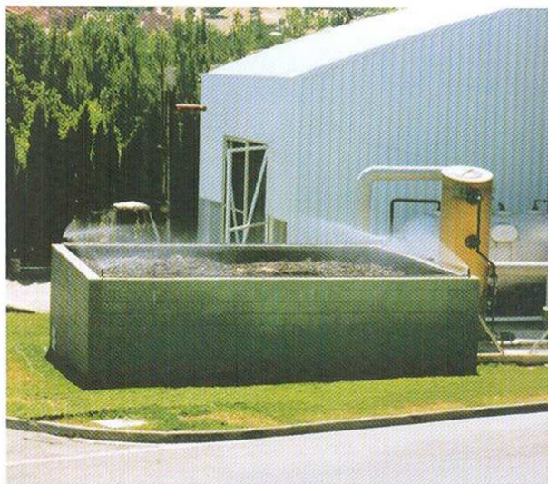
H 2 S+VOC biofiltration at a Spanish food plant 西班牙某食品厂生物法去除H 2 S+VOC
